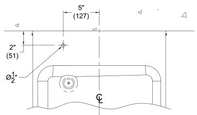
2. Drill 1/2" dia. hole thru drinking cooler deck (where shown above). Deburr hole and install grommet provided.
